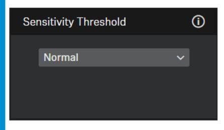
With the Microphone Sensitivity Threshold, the microphone adjusts to the background noise to better identify the speaker. Depending on the setting, the sensitivity is either amplified or attenuated.
