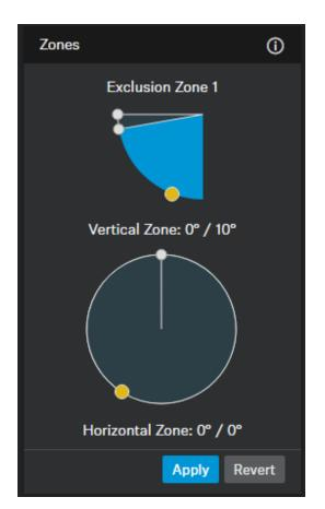
Adjust the sliders to set a vertical and horizontal zone.
