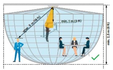
Fig. 12: Correct installation in or below the ceiling
