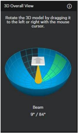
By activating the zones, 3D Overall View can displays all activated zones and current voice source in real time. The zones in the 3D model are indicated either green (prioritized) or petrol (excluded).
